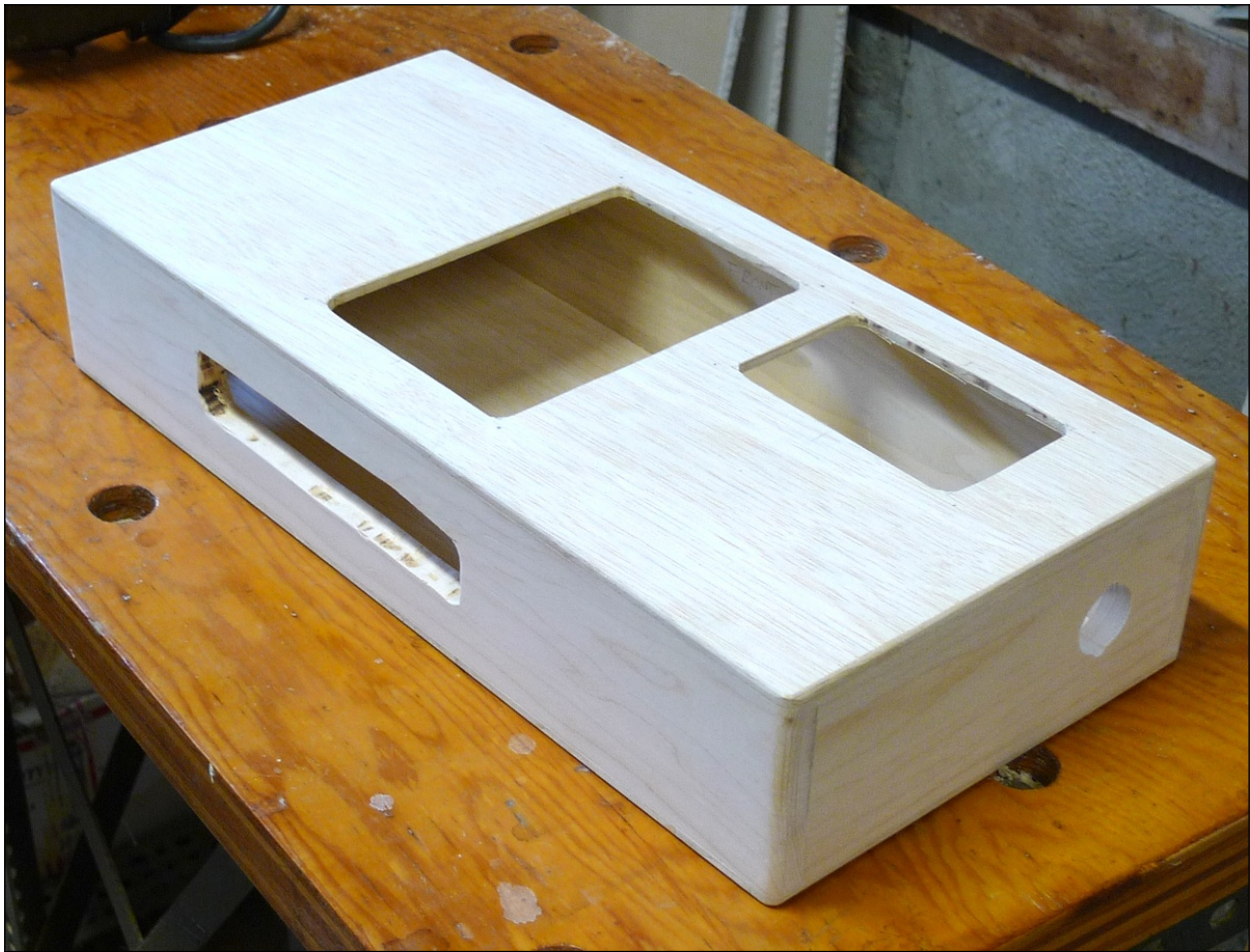
Trimmed, sanded, and routed case.
