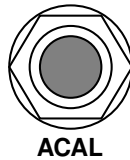
1/4" TS phone jack for ACAL external foot switch.
